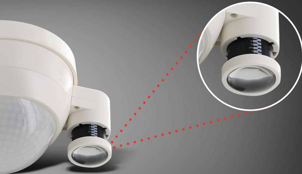
The telescopic part of the light sensor is pulled out according to the mounting height. This enables a daylight-dependant regulation to a mounting height of up to 16 m.
