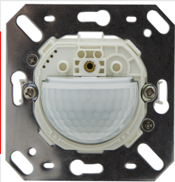
KNX PIR Wall-Mounted Motion Detector (Standard) with 180° detection angle and a range of up to 10 m (150 m 2 )
